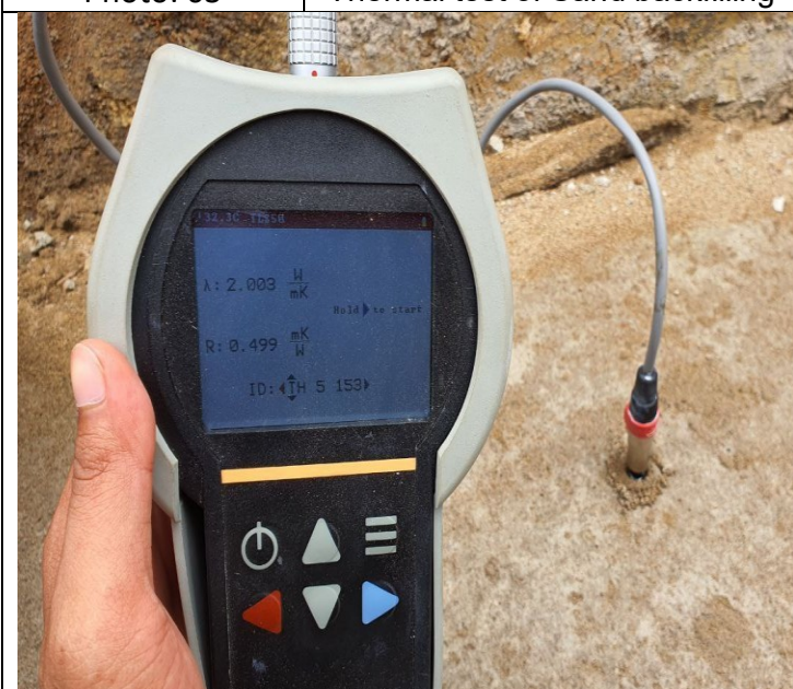
Photo: 05 Thermal test of Sand backfilling
